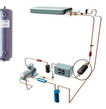
RLVCY Range Vertical liquid receivers ensure the compensation of refrigerant volume variations in refrigerating and air conditioning installations.
