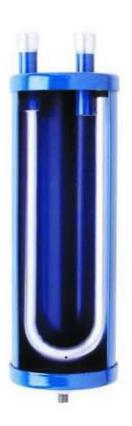
LCY Range Suction line accumlators for the elimination of risks linked to the return of refrigerant in its liquid phase and to the massive oil intake at compressor's suction of refrigerating and air conditioning installations.
