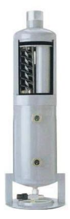
**TURBOIL-R Range** Oil separators for the separation and recovery of the oil carried by the refrigerant in vapour phase at compressor outlet of refrigerating and air conditioning installations.
